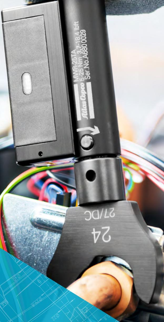
A close-up photograph of a worker's gloved hand operating an Atlas Copco MWR-25TA torque wrench. The wrench is black with a yellow ring at the handle. It is being used to tighten a bolt on a mechanical assembly. The wrench's head is marked with "24" and "27/DC". The handle has a digital display and is labeled with "MWR-25TA", "3.7-18.4 lbf ft", "Atlas Copco 5-25 Nm", and "Ser. No. A680 0029".
