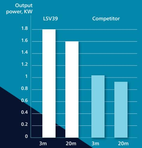
Power at different hose lengths 125 mm angle grinder.
