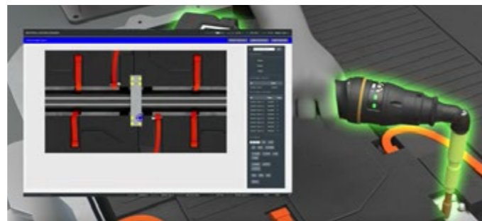
Visualized operator guidance leads the operator through the assembly process step by step
